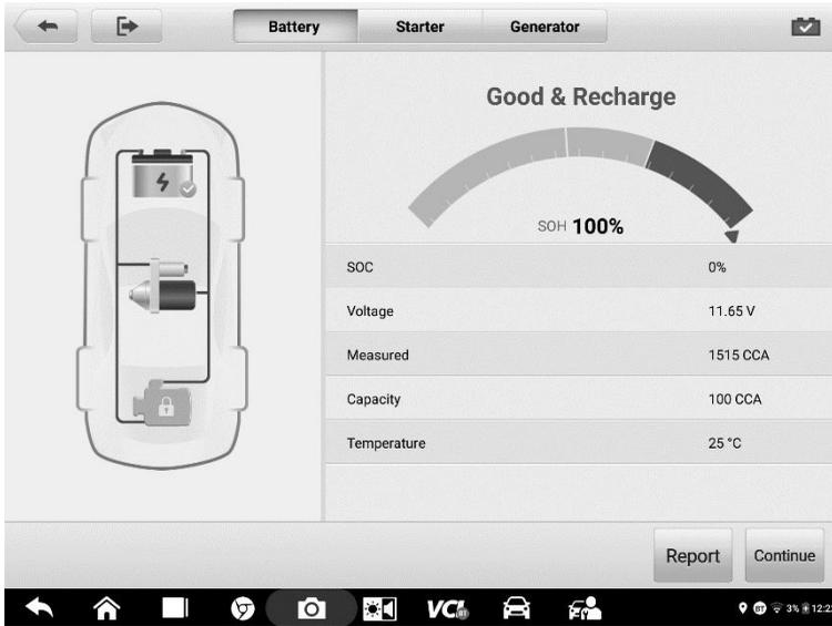
**Figure 9-4 Sample Battery Test Results Screen**
