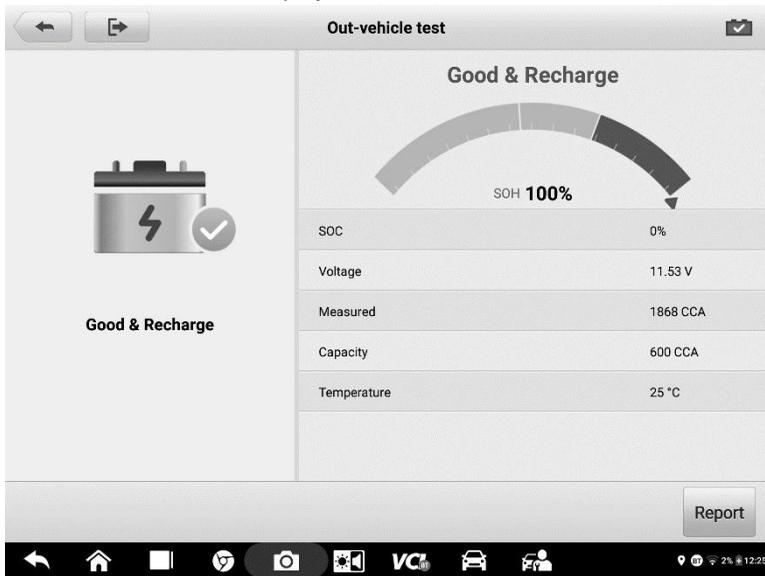
**Figure 9-8 Sample Out-vehicle Test Results Screen**
